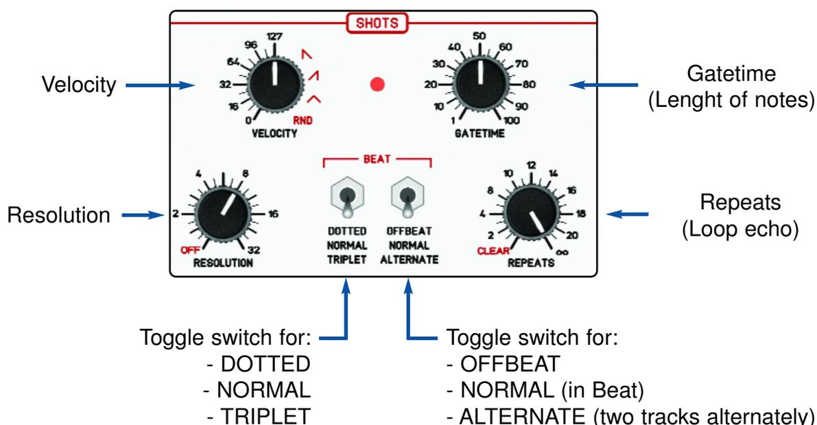
Use the knobs and buttons of the SHOTS section to set the following parameters:
