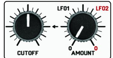
With just one AMOUNT knob, you can route both LFOs to the parameter. This also allows you to route both LFOs to the parameter at the same time. In the left third of the AMOUNT knob you only control LFO 1. In the middle third (upper part) of the AMOUNT knob both LFOs are mixed. In the right third third of the AMOUNT controller you only control LFO 2.
