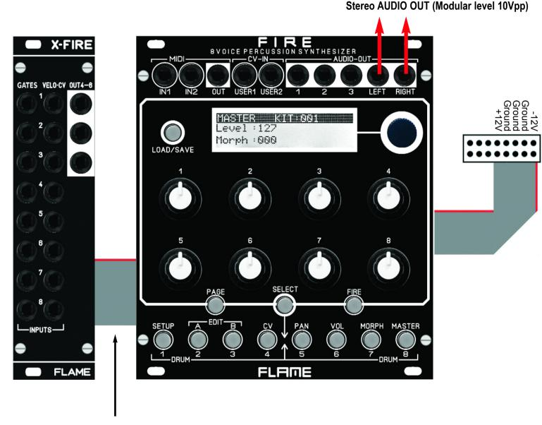
The XFIRE add-on module is connected to the basic module using the approx. 60cm long ribbon cable supplied. This additional module does not require an extra power supply.
