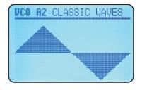
By pressing and turning the data entry knob you can switch between the wavetable name, the wave min- and max value of the selected voice in the topmost row.
