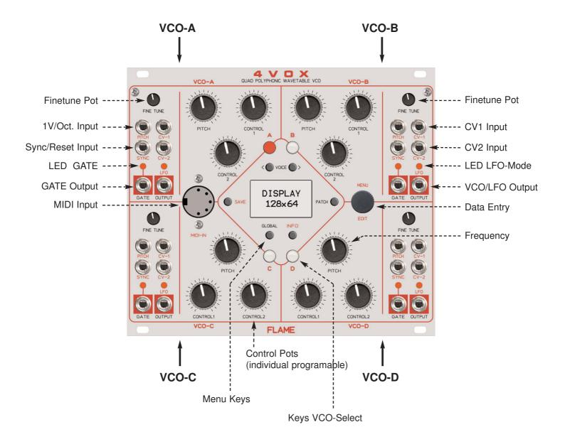
PITCH POT Pitch potentiometer Mode Analog VCO/LFO
