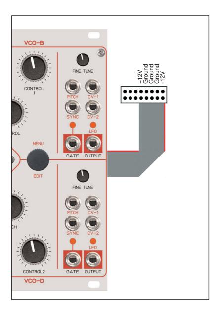
The module is delivered with a connected ribbon cable for the Doepfer bus. The red lead marks -12 volt. Connecting the module please note the right polarity!
